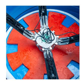
Coupled with an onboard inertial mapping unit, odometer, sonde, ultrasound, magnetic field wave, and hydrophone the Acquarius provides joint anomalies (joint gap width, axial deformation), angular
