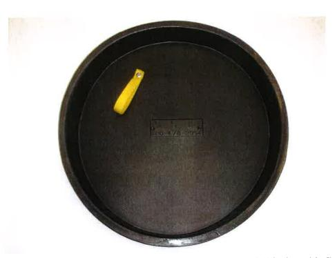
Leaking manhole covers are a major contributor to rainfall induced inflow. Sewer evaluation studies indicate that a typical manhole casting will allow an inflow rate from .20 to over 5 gallons per minute during rainfall occurrences. While the manhole cover is one of the leading contributors to collections system I & I, ironically it is the easiest and most cost-effective problem to remedy.
