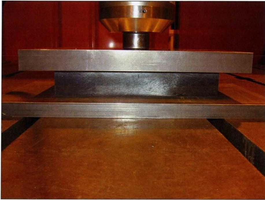
Figure 3: Compression test set-up – Example of sample installed between fixtures
