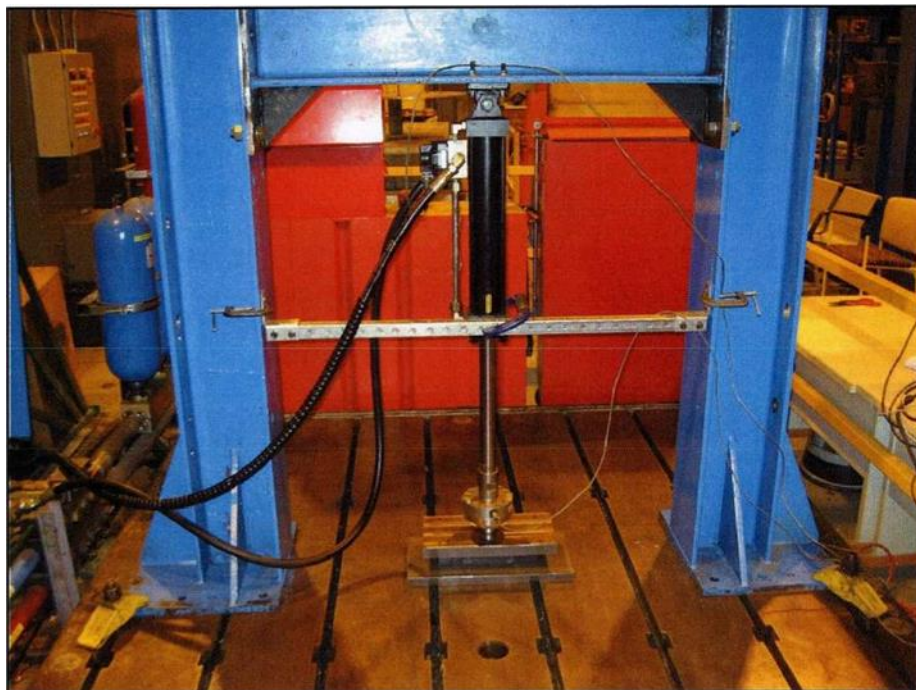
Figure 2: Compression durability test set-up – General view
