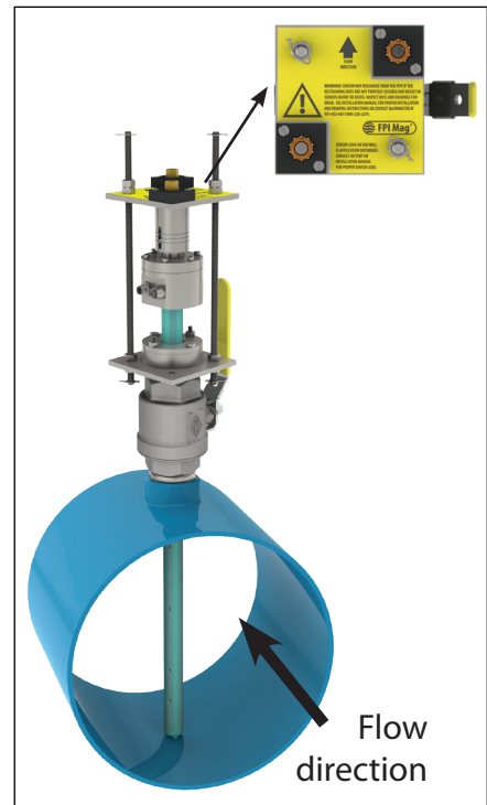
Figure 20. Meter oriented with flow direction
