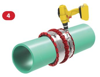
Take up all slack in coupling with a cordless drill or socket wrench. Complete the installation by tightening the tension clamps, alternating back and forth, to 80 in/lbs. minimum torque at slow speeds.
