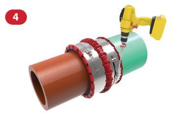
Lubricate smaller pipe end and gasket with soapy water solution. Insert pipe into coupling and take up slack with cordless drill or socket wrench. Complete installation by tightening tension clamp to 80 in/lbs. minimum torque at slow speed.
