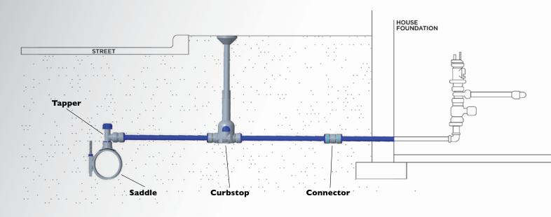
The **Megatite Tapper** and **Saddle** are supplied as a factory-assembled unit. This allows for quick and seamless installation.
