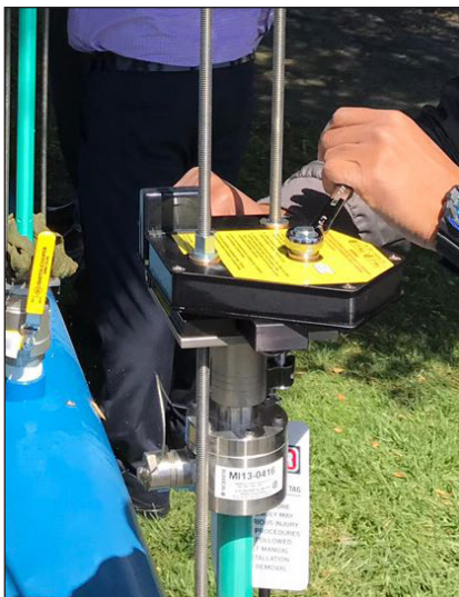
Figure 23. Inserting the sensor with the insertion tool
