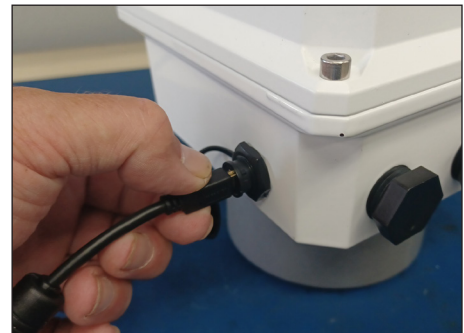
Figure 51. Plug in mini-USB cable
