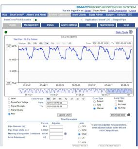
Calibration can be matched to within 1% of A/V meter results
